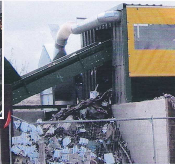
Air Knife blowing light waste back under elevator into bunker below.
